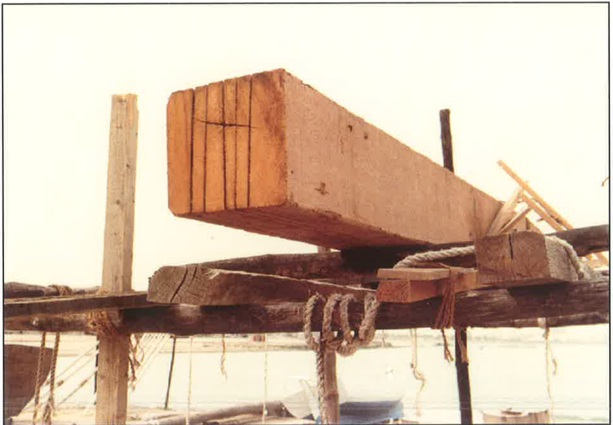
A squared-block of wood on which lines are imprinted in preparation of sawing by «al sharrah».
