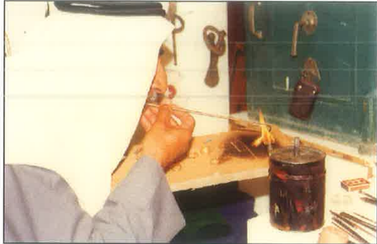
A jeweler welding a small piece of gold using «al seraj» while blowing in it through «al bori» to guide the fire towards the piece.
