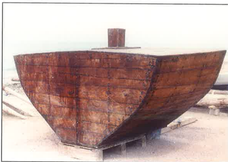
«Fintas», a wooden water tank for storing water inside the sailboat.
