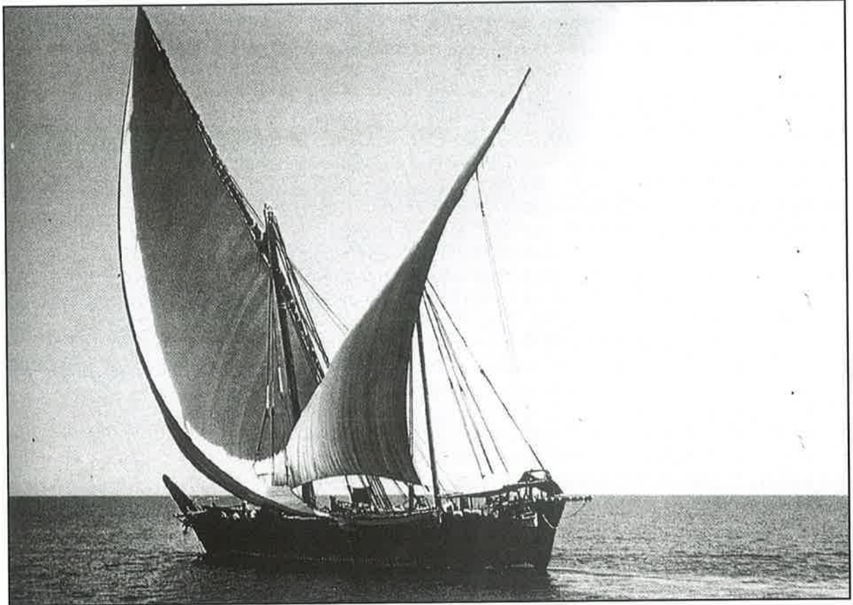
«Al Dhow» sailing with «al oad» and «al qalami» sail. It was one of the most famous Kuwaiti ships, and its load limit amounted to 6,000 maans Source: Manufacturing Sailing Ships in Kuwait, Dr. Ya'coub Yusuf Al Hijji
