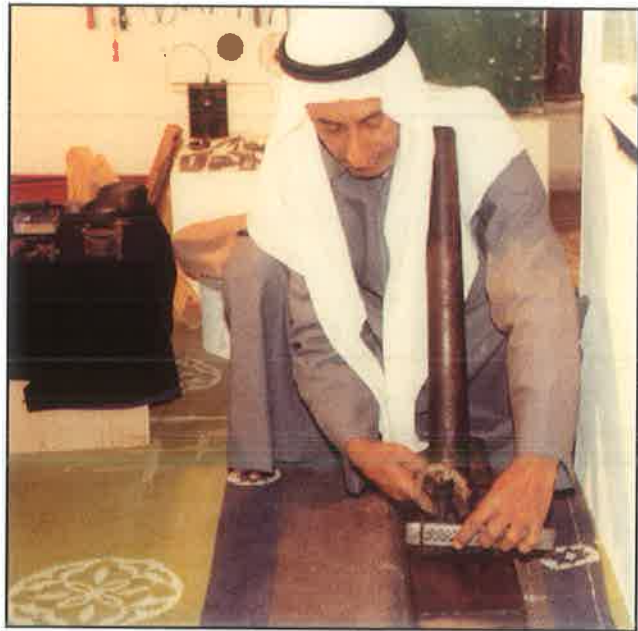
A jeweler using al mantal to pull golden wires
