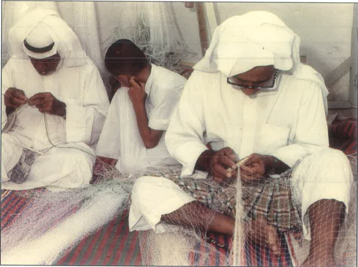
Net maker while holding «al matraqa» which determines the size of the opening of the net.
